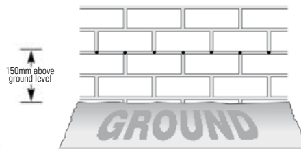
Figure 9: Drilling pattern for Stretching Bond
