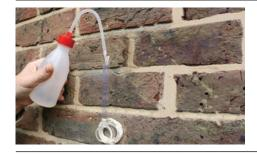
Fill the Gauge slowly with water until the water level reaches the zero mark on the Stormdry Gauge.
