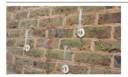
A number of Stormdry Gauges can be applied to a section of wall to identify paths of water ingress.
