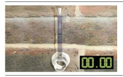
Start timing as soon as the gauge is filled. Keep a check on the water level to see if it drops. For highly absorbent surfaces this will be easily apparent within a few minutes.
