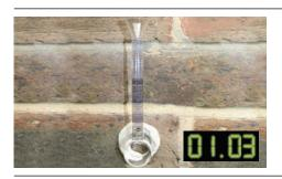
Continue to monitor the water level at regular intervals - preferably for at least one hour. The results can be plotted on a graph using the template overleaf.
